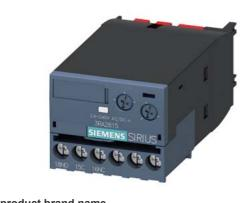
Solid-state time-delayed auxiliary switch OFF delay without control signal Relay 1 changeover contact 24...240 V AC/DC Time range 0.05...100 s Can be snapped on at the front For 3RT2 S00-S3 contactors and 3RH2 S00 contactor relays Screw terminal Varistor for attenuation of the contactor coils integrated
