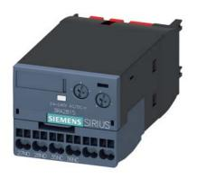
Solid-state time-delayed auxiliary switch OFF delay without control signal Relay 1 NC + 1 NO 24...240 V AC/DC Time range 0.05...100 s Can be snapped on at the front For 3RT2 S00-S3 contactors and 3RH2 S00 contactor relays Spring-type terminal Varistor for attenuation of the contactor coil integrated
