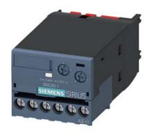
Electronic timing relay ON delay with semiconductor output 24-240 V AC/DC Time range 0.05...100 s can be snapped on at the front for contactors 3RT2 S00/S0 and auxiliary contactor 3RH2 S00 Screw terminal Varistor for attenuation of the contactor coils integrated
