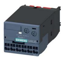
Electronic timing relay ON delay with semiconductor output 24-240 V AC/DC Time range 0.05...100 s can be snapped on at the front for contactors 3RT2 S00/S0 and auxiliary contactor 3RH2 S00 Spring-type terminal Varistor for attenuation of the contactor coils integrated
