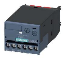
Solid-state time-delayed auxiliary switch ON delay Relay 1 changeover contact 24...240 V AC/DC Time range 0.05...100 s Can be snapped on at the front For 3RT2 S00-S3 contactors and 3RH2 S00 contactor relays Screw terminal Varistor for attenuation of the contactor coils integrated
