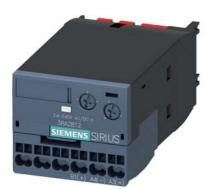
Electronic timing relay OFF delay with control signal and semiconductor output 24...240 V AC/DC Time range 0.05...100 s can be snapped on at the front for contactors 3RT2 S00/S0 and auxiliary contactor 3RH2 S00 Spring-type terminal Varistor for attenuation of the contactor coils integrated
