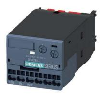
Solid-state time-delayed auxiliary switch ON delay Relay 1 changeover contact 24...240 V AC/DC Time range 0.05...100 s Can be snapped on at the front For 3RT2 S00-S3 contactors and 3RH2 S00 contactor relays Spring-type terminal Varistor for attenuation of the contactor coils integrated
