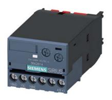
Solid-state time-delayed auxiliary switch OFF delay With control signal Relay 1 changeover contact 24...240 V AC/DC Time range 0.05...100 s Can be snapped on at the front For 3RT2 S00-S3 contactors and 3RH2 S00 contactor relays Screw terminal Varistor for attenuation of the contactor coils integrated
