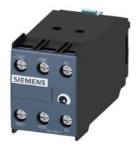
solid-state time-delayed front-side auxiliary switch Time range 0.05...1 s, 200 ... 240 V AC, 1 NO contact, 1 NC contact ON delay, for 3RT1
