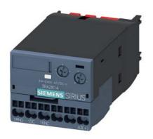
Solid-state time-delayed auxiliary switch OFF delay With control signal Relay 1 changeover contact 24...240 V AC/DC Time range 0.05...100 s Can be snapped on at the front For 3RT2 S00-S3 contactors and 3RH2 S00 contactor relays Spring-type terminal Varistor for attenuation of the contactor coils integrated
