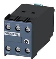
solid-state time-delayed front-side auxiliary switch Time range 0.5...10 s, 24 V AC/DC, 1 NO contact, 1 NC contact ON delay, for 3RT1
