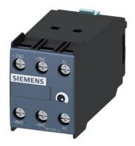
solid-state time-delayed front-side auxiliary switch Time range  $5...100~s,\,24~V$  AC/DC, 1 NO contact, 1 NC contact ON delay, for 3RT1
