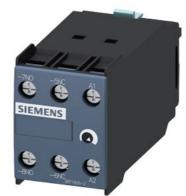
solid-state time-delayed front-side auxiliary switch Time range 0.05...1 s, 24 V AC/DC, 1 NO contact, 1 NC contact OFF delay, without control signal for 3RT1
