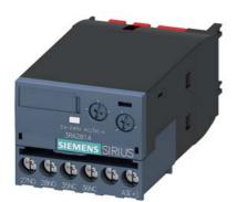
Solid-state time-delayed auxiliary switch OFF delay With control signal Relay 1 NC + 1 NO 24...240 V AC/DC Time range 0.05...100 s Can be snapped on at the front For 3RT2 S00-S3 contactors and 3RH2 S00 contactor relays Screw terminal Varistor for attenuation of the contactor coils integrated
