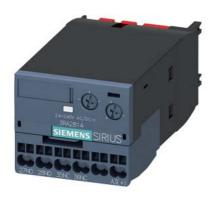
Solid-state time-delayed auxiliary switch OFF delay With control signal Relay 1 NC + 1 NO 24...240 V AC/DC Time range 0.05...100 s Can be snapped on at the front For 3RT2 S00-S3 contactors and 3RH2 S00 contactor relays Spring-type terminal Varistor for attenuation of the contactor coils integrated
