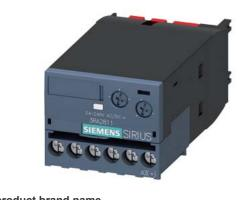
Electronic timing relay ON delay with semiconductor output 24-240 V AC/DC Time range 0.05...100 s can be snapped on at the front for contactors 3RT2 S00/S0 and auxiliary contactor 3RH2 S00 Screw terminal Varistor for attenuation of the contactor coils integrated
