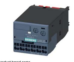
Electronic timing relay OFF delay with control signal and semiconductor output 24...240 V AC/DC Time range 0.05...100 s can be snapped on at the front for contactors 3RT2 S00/S0 and auxiliary contactor 3RH2 S00 Spring-type terminal Varistor for attenuation of the contactor coils integrated
