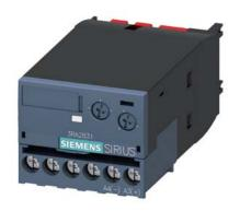
Electronic timing relay ON delay With semiconductor output 24-90 V AC/DC Time range 0.05...100 s Can be snapped on at the front For contactors 3RT2, S2, S3 and 3RH2 S00 contactor relays Screw terminal
