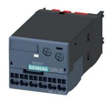
Electronic timing relay ON delay With semiconductor output 24-90 V AC/DC Time range 0.05...100 s Can be snapped on at the front For contactors 3RT2, S2, S3 and 3RH2 S00 contactor relays Spring-type terminal
