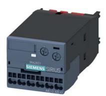
Electronic timing relay ON delay With semiconductor output 90-240 V AC/DC Time range 0.05...100 s Can be snapped on at the front For contactors 3RT2, S2, S3 and 3RH2 S00 contactor relays Spring-type terminal
