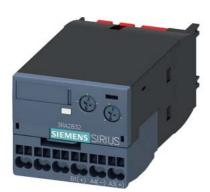
Electronic timing relay OFF delay With control signal and semiconductor output 24-90 V AC/DC Time range 0.05...100 s Can be snapped on at the front For contactors 3RT2, S2, S3 and 3RH2 S00 contactor relays Spring-type terminal
