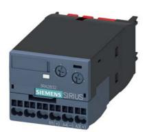
Electronic timing relay OFF delay With control signal and semiconductor output 90-240 V AC/DC Time range 0.05...100 s Can be snapped on at the front For contactors 3RT2, S2, S3 and 3RH2 S00 contactor relays Spring-type terminal
