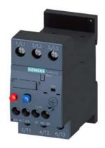
Overload relay 27...32 A Thermal For motor protection Size S0, Class 10 Stand-alone installation Main circuit: Screw Auxiliary circuit: Screw Manual-Automatic-Reset
