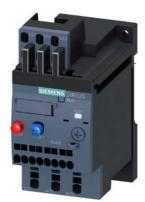
Overload relay 1.8...2.5 A Thermal For motor protection Size S00, Class 10 Stand-alone installation Main circuit: Spring-type terminal Auxiliary circuit: spring-type terminal Manual-Automatic-Reset
