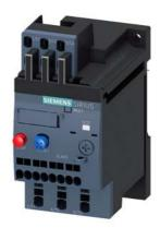
Overload relay 7.0...10 A Thermal For motor protection Size S00, Class 10 Stand-alone installation Main circuit: Spring-type terminal Auxiliary circuit: spring-type terminal Manual-Automatic-Reset
