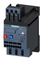
Overload relay 1.1...1.6 A Thermal For motor protection Size S00, Class 10 Stand-alone installation Main circuit: Spring-type terminal Auxiliary circuit: spring-type terminal Manual-Automatic-Reset
