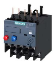
Overload relay 9.0...12.5 A Thermal For motor protection Size S00, Class 10 Contactor mounting Main circuit: Ring cable lug Auxiliary circuit: ring cable lug Manual-Automatic-Reset
