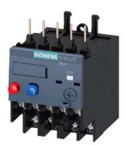
Overload relay 11...16 A Thermal For motor protection Size S00, Class 10 Contactor mounting Main circuit: Ring cable lug Auxiliary circuit: ring cable lug Manual-Automatic-Reset
