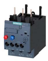
Overload relay 4.5...6.3 A Thermal For motor protection Size S0, Class 10 Contactor mounting Main circuit: Screw Auxiliary circuit: Screw Manual-Automatic-Reset
