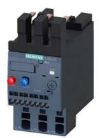
Overload relay 4.5...6.3 A Thermal For motor protection Size S0, Class 10 Contactor mounting Main circuit: Spring-type terminal Auxiliary circuit: spring-type terminal Manual-Automatic-Reset
