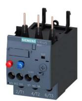
Overload relay 9.0...12.5 A Thermal For motor protection Size S0, Class 10 Contactor mounting Main circuit: Screw Auxiliary circuit: Screw Manual-Automatic-Reset
