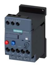
Overload relay 1.4...2.0 A Thermal For motor protection Size S00, Class 10 Stand-alone installation Main circuit: Screw Auxiliary circuit: Screw Manual-Automatic-Reset
