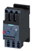
Overload relay 23...28 A Thermal For motor protection Size S0, Class 10 Stand-alone installation Main circuit: Spring-type terminal Auxiliary circuit: spring-type terminal Manual-Automatic-Reset
