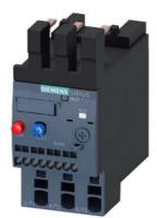
Overload relay 30...36 A Thermal For motor protection Size S0, Class 10 Contactor mounting Main circuit: Spring-type terminal Auxiliary circuit: spring-type terminal Manual-Automatic-Reset
