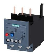
Overload relay 5.5...8 A Thermal For motor protection Size S2 Class 10 Contactor mounting Main circuit: screw terminal Auxiliary circuit: screw terminal Manual-Automatic-Reset
