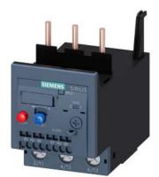
Overload relay 7...10 A Thermal For motor protection Size S2 Class 10 Contactor mounting Main circuit: screw terminal Auxiliary circuit: springtype terminal Manual-Automatic-Reset
