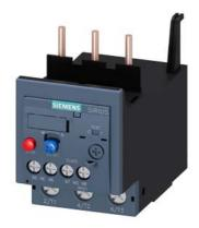
Overload relay 11...16 A Thermal For motor protection Size S2, Class 10 Contactor mounting Main circuit: Screw Auxiliary circuit: Screw Manual-Automatic-Reset
