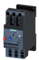
Overload relay 34...40 A Thermal For motor protection Size S0, Class 10 Stand-alone installation Main circuit: Spring-type terminal Auxiliary circuit: spring-type terminal Manual-Automatic-Reset
