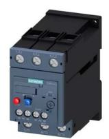
Overload relay 40... 50 A Thermal For motor protection Size S2, Class 10 Stand-alone installation Main circuit: Screw Auxiliary circuit: Screw Manual-Automatic-Reset
