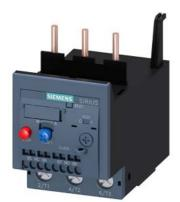
Overload relay 54...65 A Thermal For motor protection Size S2, Class 10 Contactor mounting Main circuit: Screw Auxiliary circuit: spring-type terminal Manual-Automatic-Reset
