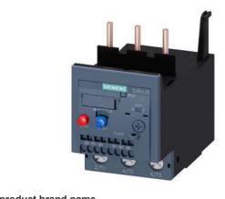
Overload relay 47...57 A Thermal For motor protection Size S2, Class 10 Contactor mounting Main circuit: Screw Auxiliary circuit: spring-type terminal Manual-Automatic-Reset
