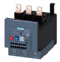
Overload relay 36...50 A Thermal For motor protection Size S3, Class 10 Contactor mounting Main circuit: Screw Auxiliary circuit: spring-type terminal Manual-Automatic-Reset
