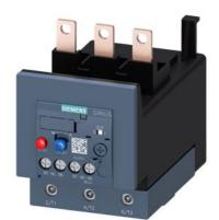
Overload relay 45...63 A Thermal For motor protection Size S3, Class 10 Contactor mounting Main circuit: Screw Auxiliary circuit: Screw Manual-Automatic-Reset
