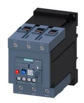
Overload relay 57...75 A Thermal For motor protection Size S3, Class 10 Stand-alone installation Main circuit: Screw Auxiliary circuit: Screw Manual-Automatic-Reset
