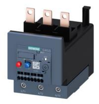
Overload relay 57...75 A Thermal For motor protection Size S3, Class 10 Contactor mounting Main circuit: Screw Auxiliary circuit: spring-type terminal Manual-Automatic-Reset
