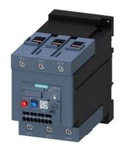
Overload relay 57...75 A Thermal For motor protection Size S3, Class 10 Stand-alone installation Main circuit: Screw Auxiliary circuit: spring-type terminal Manual-Automatic-Reset
