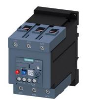
Overload relay 70...90 A Thermal For motor protection Size S3, Class 10 Stand-alone installation Main circuit: Screw Auxiliary circuit: Screw Manual-Automatic-Reset
