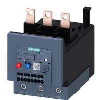
Overload relay 70...90 A Thermal For motor protection Size S3, Class 10 Contactor mounting Main circuit: Screw Auxiliary circuit: spring-type terminal Manual-Automatic-Reset
