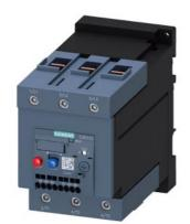
Overload relay 70...90 A Thermal For motor protection Size S3, Class 10 Stand-alone installation Main circuit: Screw Auxiliary circuit: spring-type terminal Manual-Automatic-Reset
