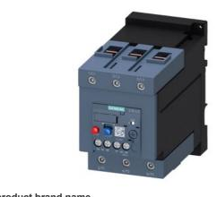
Overload relay 80...100 A Thermal For motor protection Size S3, Class 10 Stand-alone installation Main circuit: Screw Auxiliary circuit: Screw Manual-Automatic-Reset
